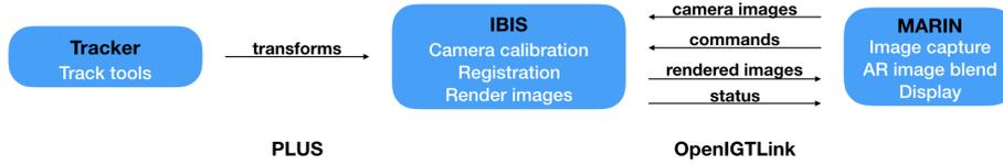
**Fig. 2** Block diagram representing interactions between system components and data flow.
