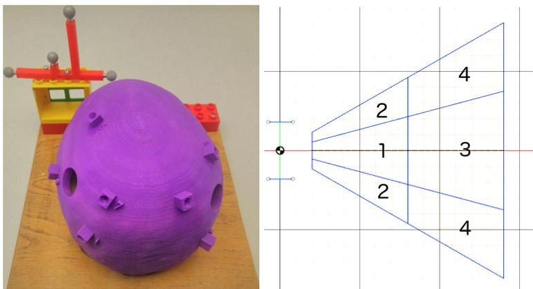
**Fig. 4** Experimental phantom design. On the left: the phantom seen from the back, with craniotomies on either side, fiducials and the marker behind. On the right: a depiction of the four difficulty zones used in the experiment. The craniotomy is located between the two blue lines on the left and is centered on the dot. Then the four zones are: 1:  $0-15^\circ$  from normal, 1-4 cm deep; 2:  $15-30^\circ$ , 1-4 cm; 3:  $0-15^\circ$ , 4-7 cm; 4:  $15-30^\circ$ , 4-7 cm.
