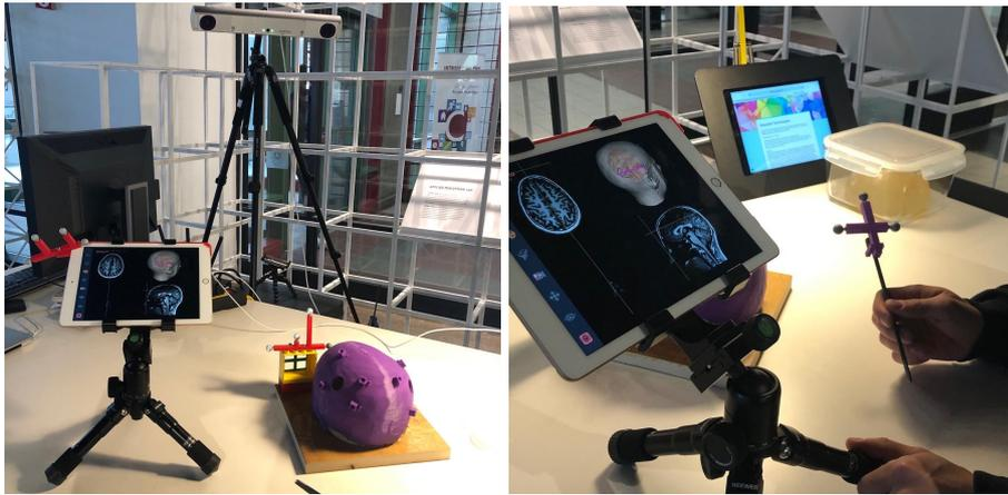
**Fig. 1** Photos of the system, as was used in test study described in section 4. On the left: the iPad running MARIN mounted on an adjustable tripod, the phantom and the tracking system mounted on a larger immovable tripod at the back, behind the table. On the right: the iPad running MARIN and the tracked pointer.
