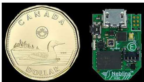
Figure 2: The Neblina™ motion sensor compared to a Canadian one-dollar coin size-wise.
